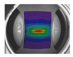
The AutoGrid<sup>®</sup> product family enables for strain analysis on samples and components in sheet metal industry. It proved well suited for a variety of applications in deep drawing and hydroforming as well as for different materials including aluminium alloys, stainless steel, and fibre reinforced composites.
