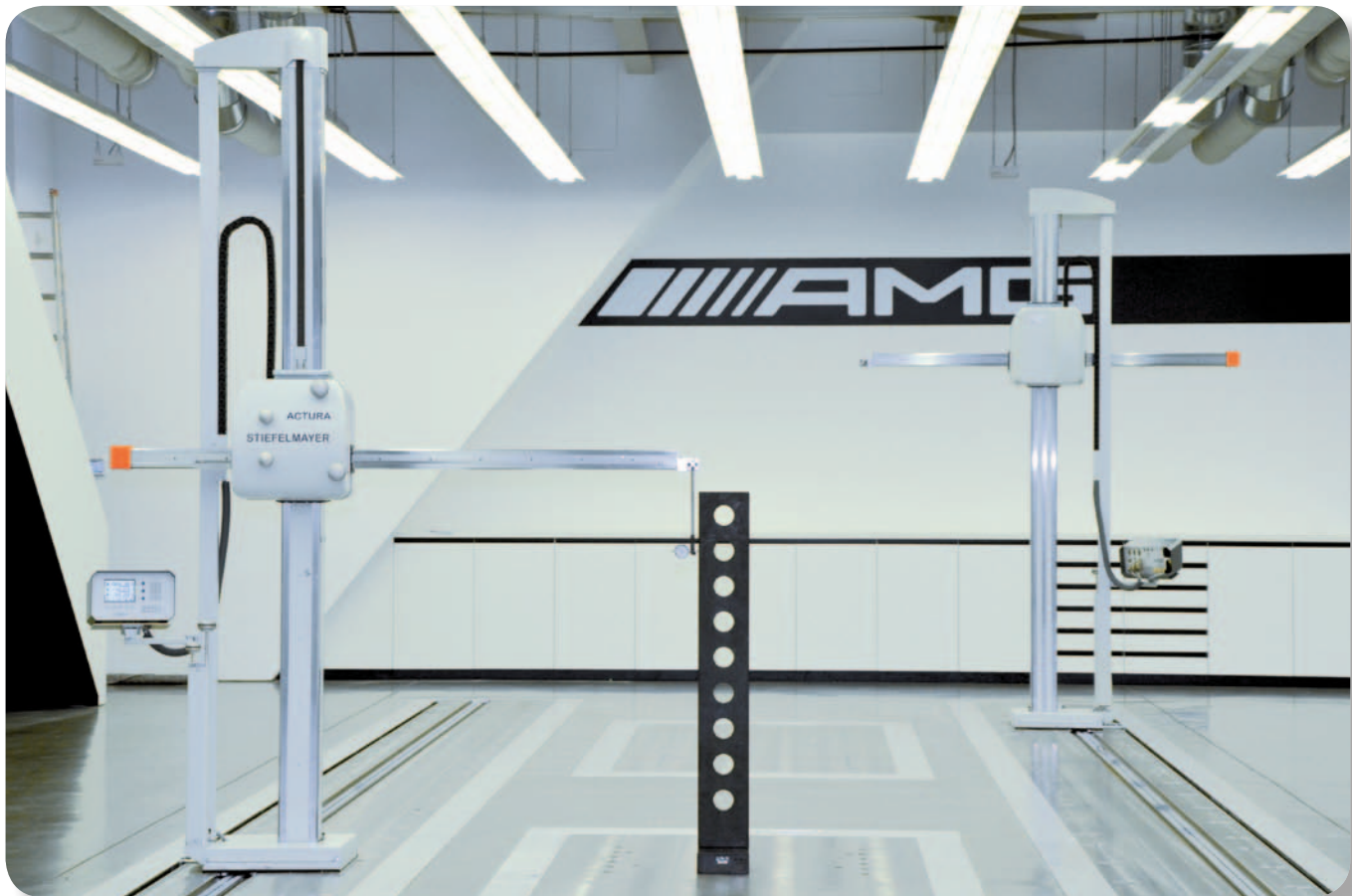
Duplex ACTURA, with several single measuring plates installed between the guide beams.
