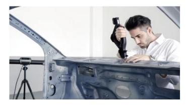
It can be paired with a portable CMM T-Probe (optional with different sizes) to probe inaccessible areas such as holes and hidden points. This contact measurement probe can ensure precise results with high single-point repeatability of 0.030 mm.
