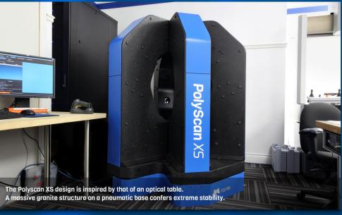
Our SURROUND 3D SCANNERS™ are by design immobile during the inspection. This makes them safe and simple to operate: place a part in the center and press Scan. Their unique calibration avoids the need for data alignment and their multiple baselines increase accuracy when measuring points.
