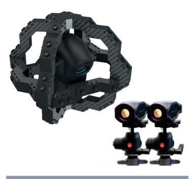
The Metronor cameras automatically track the LEDs on each side of the scanner frame, no matter its orientation
